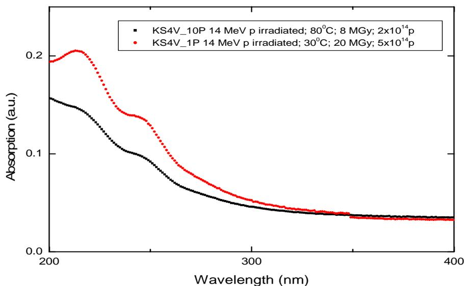
*Figure 3 KS-4V absorption spectra - comparison between 14 MeV p irradiation at 30°C to 20 MGy and 14 MeV p irradiation at 80°C to 8 MGy*
