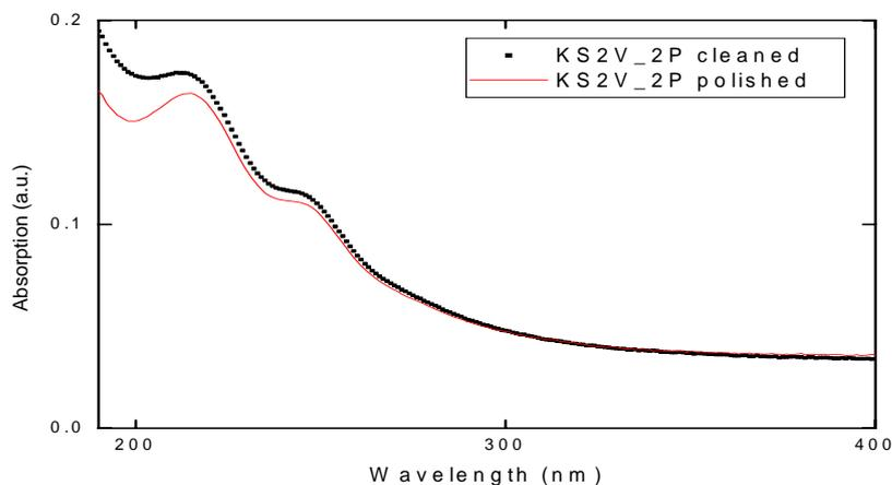
*Figure 4 Absorption spectra on KS-4V sample 14 MeV p irradiated at 30 °C to 16 MGy - before and after polishing*
